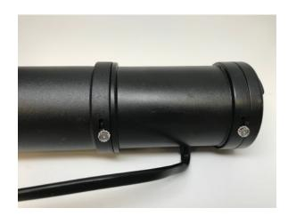
On the back of the main unit, locate the 2 clear plastic pins. These pins hold the unit together and ensure that potentially harmful UV rays remain inside the unit. With the help of a tool, (pliers or tweezers work fine) firmly grasp the pin, rotate, and pull outward to remove. (The pin is not threaded, but it does fit snugly.) Take care not to lose these pins, because you will need them to reassemble unit.
